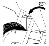
**2** Locate fuse cover on top of battery assembly through the rear fender.
